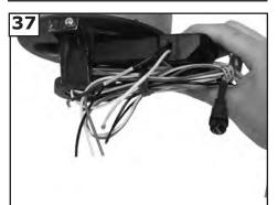
Slide remote receiver into mounting bracket.
